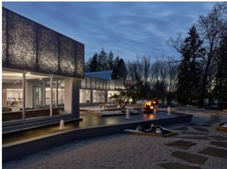
Translucent aluminum foam panels framing 25-foot-tall LED video wall at EarthCam's new headquarters
