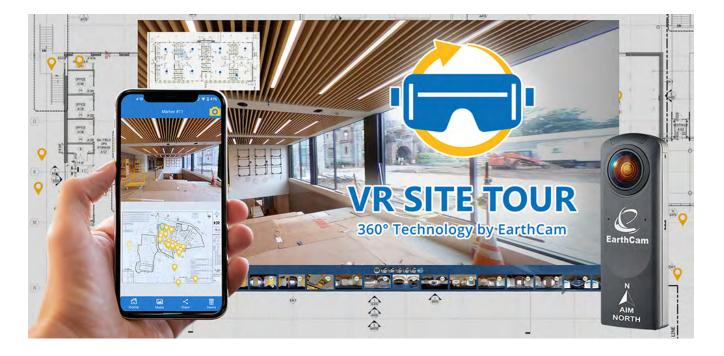
VR Site Tour interactive images are captured using a standard 360° camera, combined with EarthCam's environmental sensor data, and automatically assembled into a virtual project tour.
